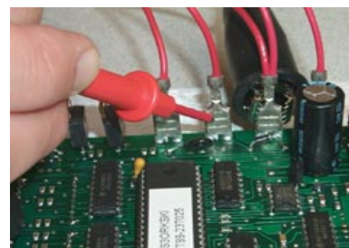
Measuring Controller Voltage
