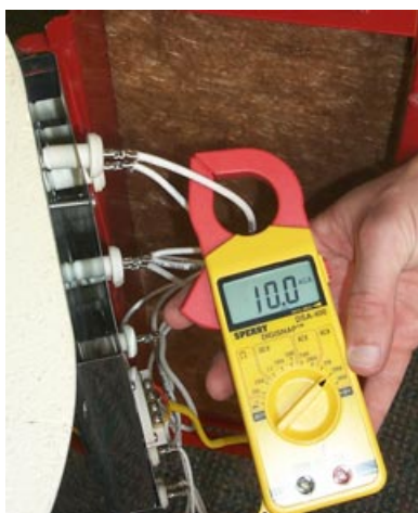
Testing Amperage at Feeder Wires
