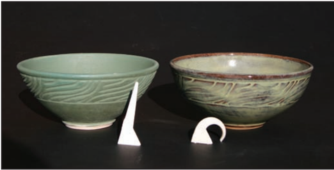
Pyrometric cones help you understand possible glaze problems. ^ The cone on the left is erect and under-fired, explaining why the glaze surface has a dry, rough and matte finish. The cone and pot on the right show a good firing and the same glaze has matured to a glossy surface on a slightly darker clay body.
