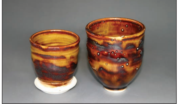
Two test pots, both fired to glaze maturity: Left clay body and glaze are OK. Right pot still had organic matter that was not totally burnt off during the bisque firing, thus it escaped in the glaze firing, causing pinholes and blisters in the glaze surface as it was released from the clay body. The solution to this problem is a longer/slower bisque firing to help burn out all the organic matter.
