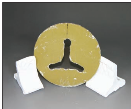
This simple die was made to extrude test tiles that were cut into 1- to 1.5-inch sections.
